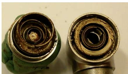
Fig. 2: Head unit of a transmission instrument. Deposits and corrosion in tongs due to unsuitable reprocessing methods (Photo: Sirona)
