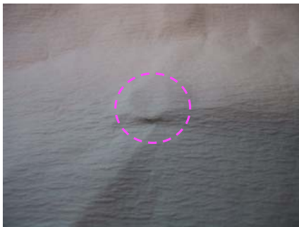
damaged paper caused by nuts sticking out
